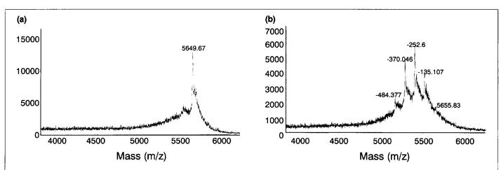
**Figure 4.** Detection of abasic sites in DNA by MALDI-TOF-MS. (a) Spectrum obtained for synthetic 19 nucleotide DNA purified by automated solid-phase extraction. Theoretical mass, 5650, obtained, 5649.67. (b) Spectrum obtained for the same oligonucleotide after treatment at pH 1.75 for 18 h at room temperature.
