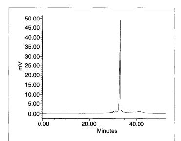
**Figure 3.** Capillary electropherogram of a 25 nucleotide DNA purified by automated solid-phase extraction.
