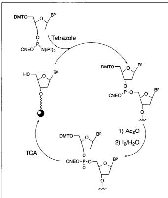
**Figure 1.** Solid-phase DNA synthesis cycle using the phosphoramidite approach. DMT, dimethoxytrityl; CNE, cyanoethyl;  $B^p$ , exocyclic amino protected base; iPr, isopropyl;  $Ac_2O$ , acetic anhydride; TCA, trichloroacetic acid.
